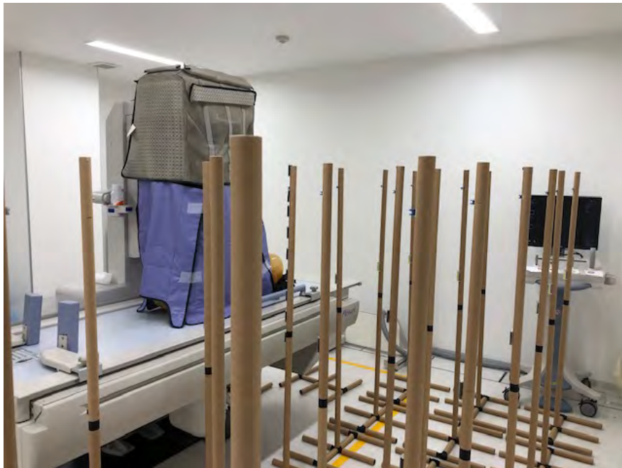
Fig. 2 Photograph for measuring the ambient dose (a) and the air kerma along height direction (b).
